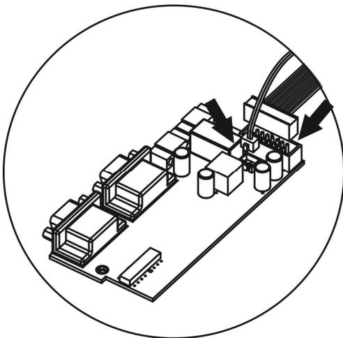
**Step 6:** Put wire cover back to the unit. Now the inverter is providing parallel operation function.
