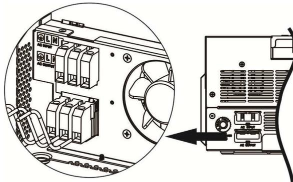
5. Make sure the wires are securely connected.
