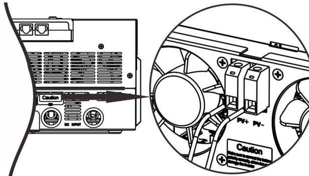
3. Make sure the wires are securely connected.
