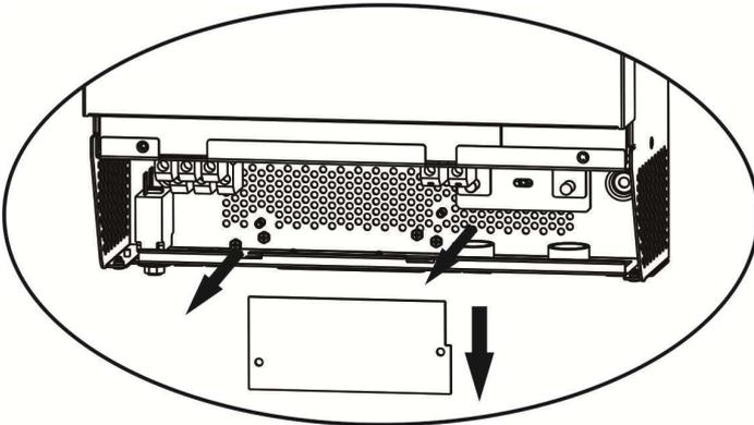
**Step 3:** Remove two screws as below chart to take out cover of parallel communication.
