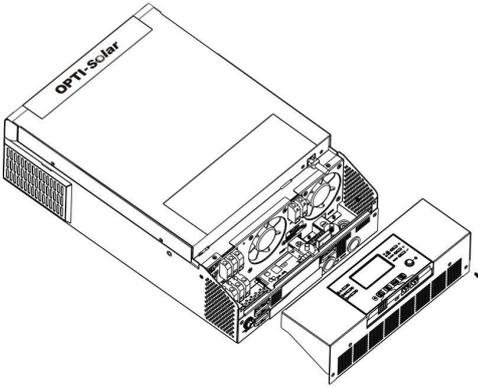
**Step 2:** Remove two screws as below chart and remove 2-pin and 14-pin cables.
