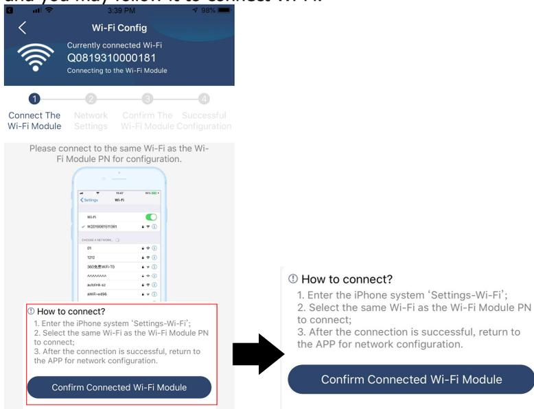
Enter the "Settings→Wi-Fi" and select connected Wi-Fi name. The connected Wi-Fi name is the same to your Wi-Fi PN number and enter default password "12345678".
